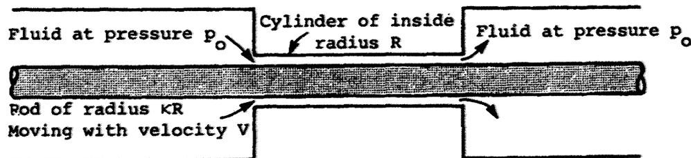
Using the continuity equation and the equation for motion, obtain expressions for the velocity distribution and the volumetric flow rate.
