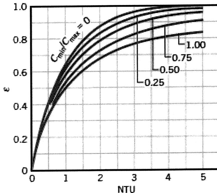
**Counterflow Heat Exchanger Performance: Effectiveness Factor (ε) vs. Number of Transfer Units (NTU) for Various C<sub>min</sub>/C<sub>max</sub> Ratios**
